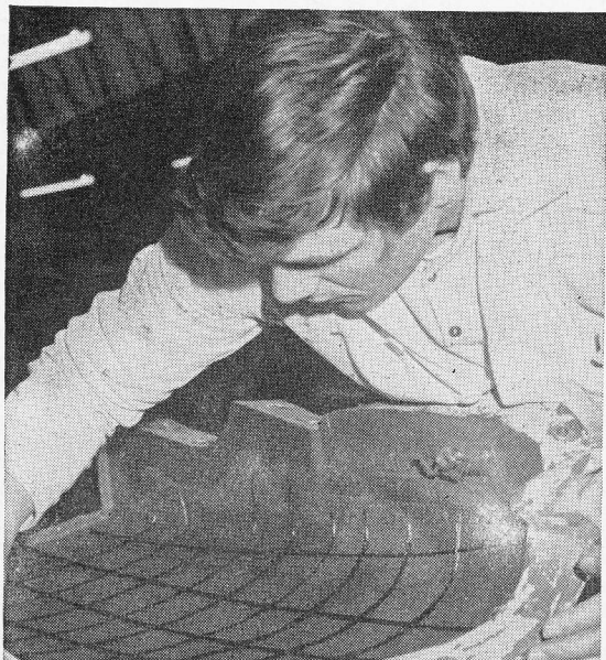
Carbon filaments are lined inside a Lola GT body (left). These recently-introduced filaments give added strength with less weight. In one of the prototype bays (right) work is taking place on the Chevron B16. The full-size "Datum" bridge slides to and fro on rails for measurements to be taken from all angles.
